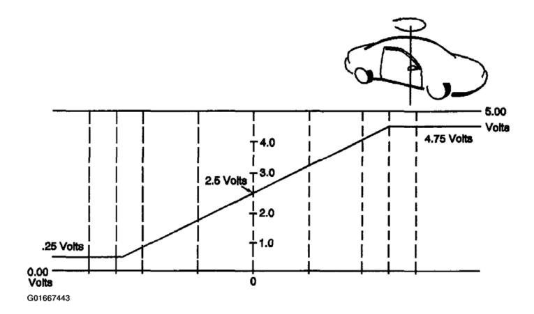
Yaw Rate Sensor - Voltage Chart Courtesy of GENERAL MOTORS CORP. .
